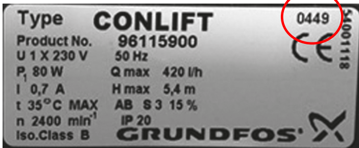
Figure 2 – Showing an example of the data badge where the month and year of manufacture are highlighted within the red circle.
