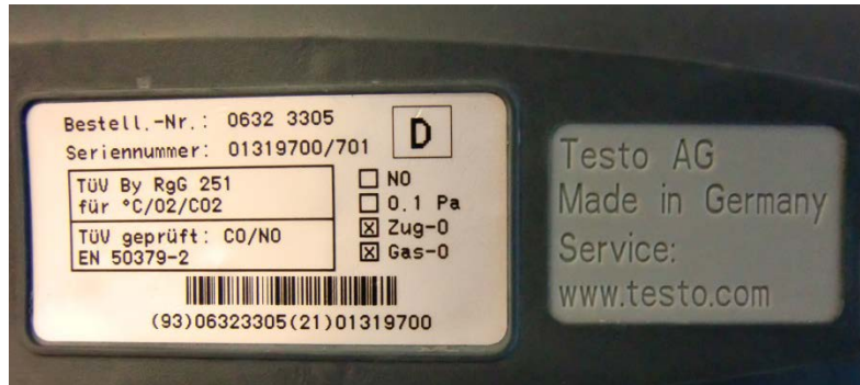
Figure 1 – Showing the specification plate on the rear of the instrument (check [Bestell Nr] against numbers of affected instruments as given in Table1 ).
